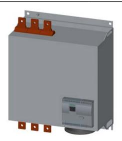
SIRIUS SOFT STARTER, VALUES AT 460V, 50DEGREES, STANDARD: 850A, 750HP, INSIDE-DELTA CIRCUIT 3: 1472A, 1300HP, AC 200-460V, AC 115V, SCREW TERMINALS
